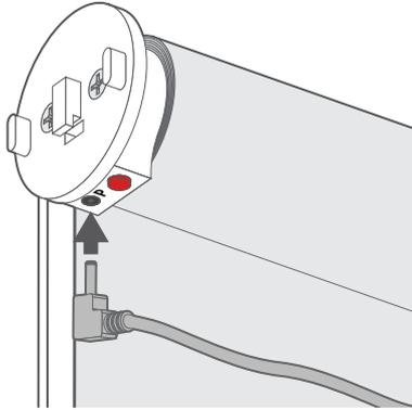
To charge the battery, plug the charger cable into the charging port on the motor.
