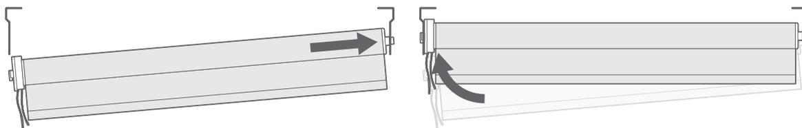
Locate the depression end (the opposite end to the controls) of the blind into the circular hole in the corresponding bracket. Lift the control end of the blind and slot the rectangular 'lugs' into the corresponding slots on the bracket.
