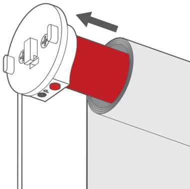
If you do not have a plug socket close enough for the charger cable to reach, then the motor can be easily removed from the roller tube to make charging easier.
