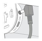
Once your blind is installed we recommend plugging in the motor to allow it to fully charge before use.
