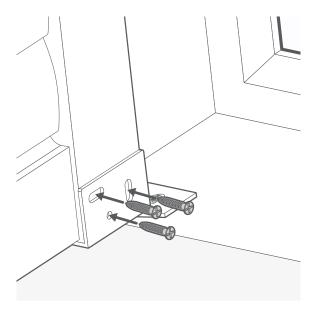
Hold the shutters up against the hinges and screw them into place using 3x 18.5mm screws per hinge.
