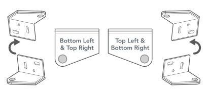
Note that there is a 'left' and 'right' version of each hinge, so they should be placed in the window accordingly.
