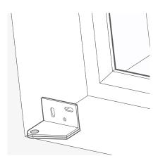
Swing the hinge open to access the screw holes more easily.
