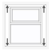
Fit 1 hinge into each corner of the window, top and bottom.
