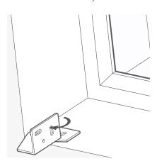
Use 2x 18.5mm screws per hinge to fix it into the recess.
