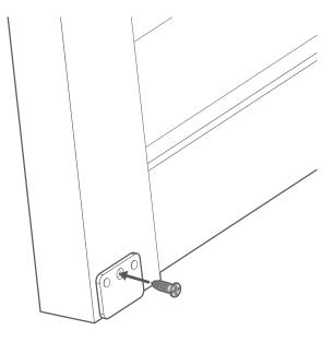
Finally, attach the metal strike plates to the back of the shutter panels, so that they're in line with the magnets. Use 1x 12mm screw per plate.
