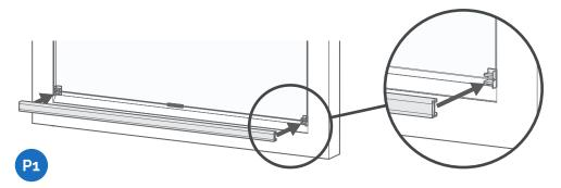
To finish, clip the bottom rail into the lower brackets by aligning the rail with the brackets and pushing back firmly towards the glass, until the rail clicks into place.
