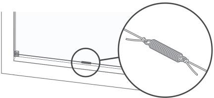
At the bottom of the blind the cord is connected to both ends of a small spring. Until the knot at one side of the spring.
