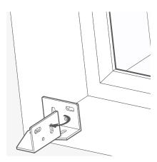
Use 2x 18.5mm screws per hinge to fix it into the recess.
