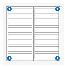
If your order contains more than 2 panels, install the outer panels first. Then fit the hinges for the centre panel 3mm away from the edge of its neighbouring panel.
