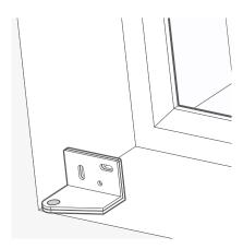
Swing the hinge open to access the screw holes more easily.
