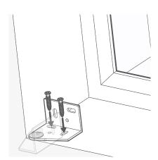
Each panel is supplied with 2 hinges. If your order contains only 1 panel then install the hinges on the side you requested when ordering.
