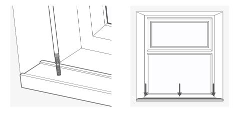
Next, install the top channel in the same way. Start with the centre screw so that the channel is supported while you screw in the others. Space your screws in the same way as you did for the bottom channel.
