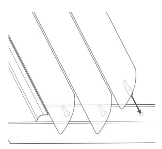
Rest the panel on its side and slot the louvres into place, locating the back half of each louvre pin into its corresponding hole on the stile.
