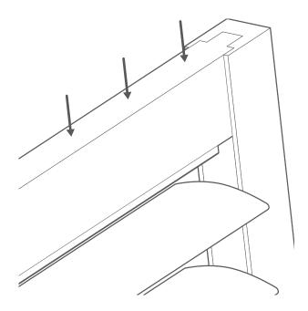
Straighten the panel and slot the top bar into place.
