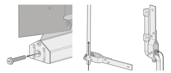
Unscrew and remove the hex nuts from the ends of the bottom bar and put them safely to one side for now. Take the side runners and feed them onto the bottom of the guide bars, then slide them up until they turn and face vertical, near the top of the guide bars.
