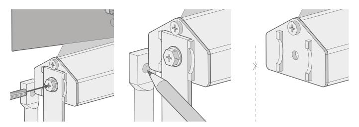
Attach the guide runners to the ends of the bottom bar using the hex nuts you removed. Hold the guide bars up against the wall, as close to the underside of the blind's cassette as possible, and mark the position of the screw holes in the guide bars. You now have an accurate centre line for the guide bar screw holes.
