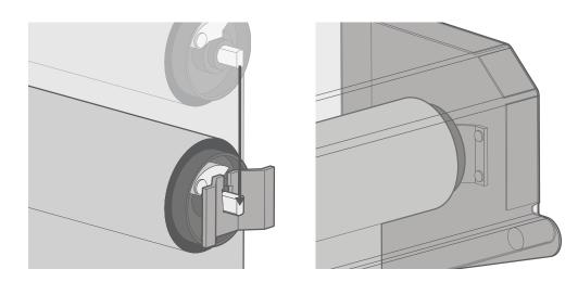
Lift the blind up into the cassette and slot the spring pin into the plate on the inside of the cassette. Be careful not to turn the blind as you do so, as this may allow the locking latch to drift into its unlocked position and release the tension in the spring mechanism.
