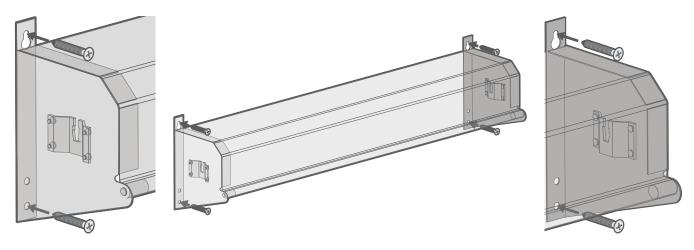
Use the top and bottom screw holes on the back of the cassette to face-fix the cassette to the wall.
