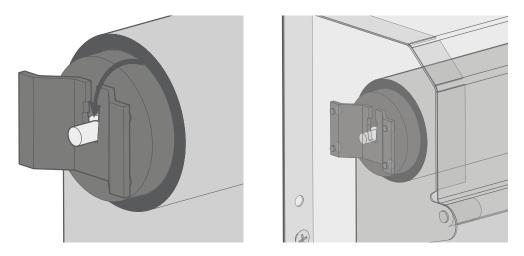
Lift the other blind into place and slot the roller pin into the other plate.
