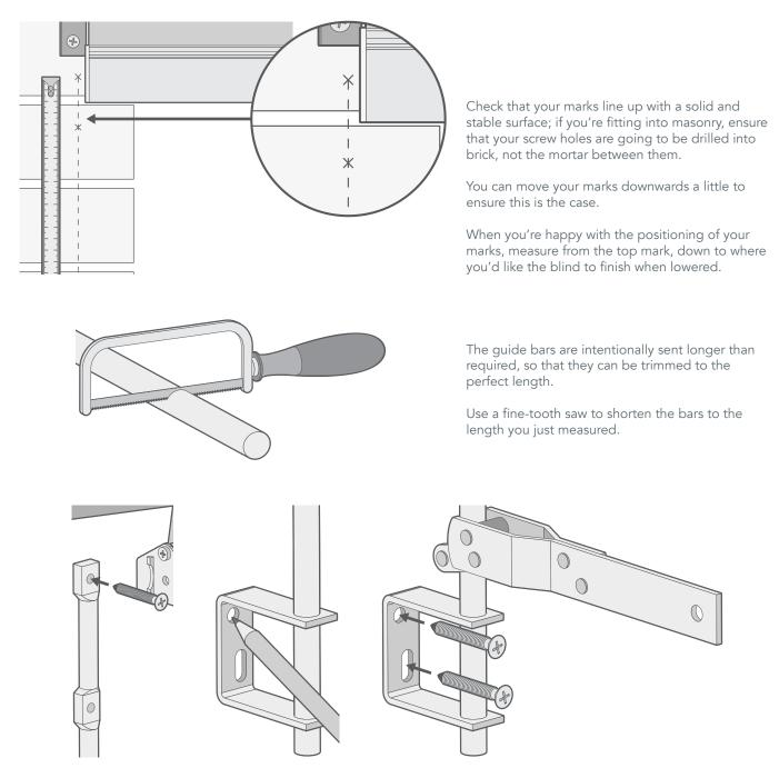
Use a hammer drill to make screw holes where you made your final marks, then fit the bars in place using the plugs and screws provided. Fit just the top screw for now, loosely enough that the bar can swing from side to side at the bottom.
