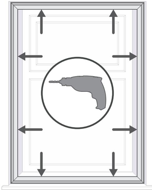
Making sure that the frame stays still and level, push the drill through each of the fixing holes you made in the frame and drill a small pilot hole in the surface you're fixing the shutter to (the inside of the recess). Drill through the plaster as far as the timber beneath. You should now be left with shallow pilot holes all around the recess - two for each side, the top and the sill.
