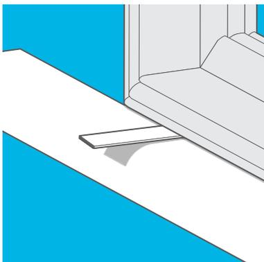
If you need to adjust the level of the frame then you can use the frame shims from your fitting kit. Fully insert the shim so that it is hidden by the frame.
