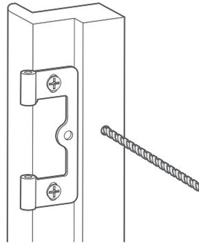
For 'Front of Recess' fitting, drill through the thicker section toward the back of the frame.
