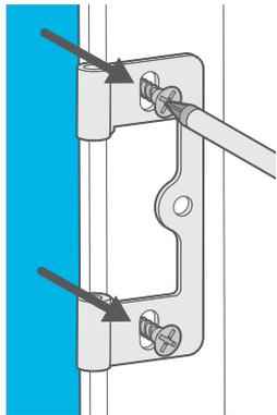
Start by loosening the frame hinges, as this will make aligning the two parts of the hinge easier (one part is fixed to the frame, the other part is fixed to the panel). This will also allow you enough room to slot the hinge pins into place.
