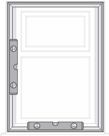
Place the assembled frame in the recess and use a spirit level to make sure that it is sitting perfectly straight on all sides.
