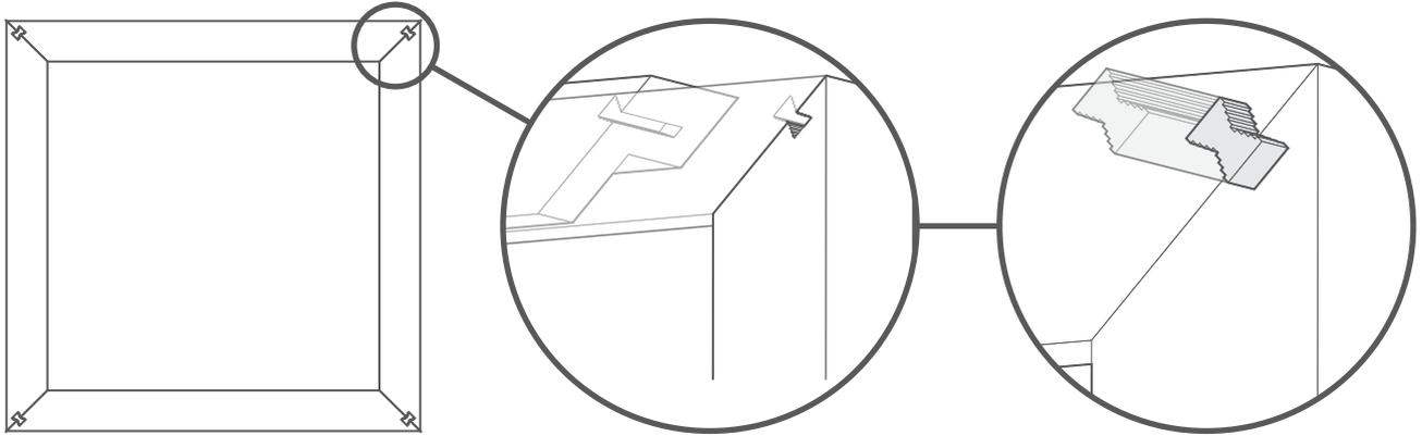
Line up all the corners, then insert the Hoffman keys from your fittings kit to join the frames securely together. The key can be a little tight, so you may have to give it a few taps with a hammer to fully insert it.
