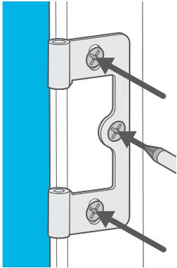
Tighten the hinge screws and insert a final screw in the centre hole for each frame hinge, to lock the hinges in place.
