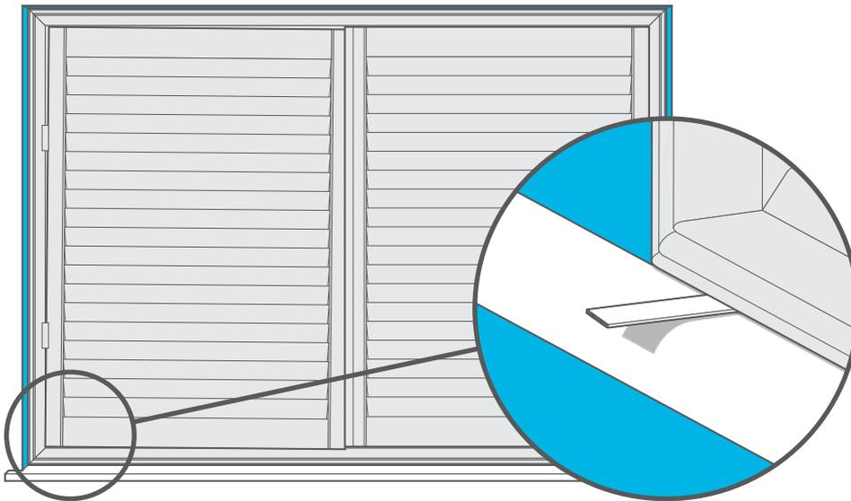
The best method for adjusting the level of the panels is actually to adjust the frame. If one panel sits higher than the other, go to the side which is sitting lowest and loosen the frame screws on that side, and along the bottom. Then insert one of the frame shims from your fixing kit to raise that side slightly. This should level out the panels.
