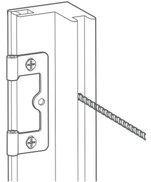
For 'Inside Recess' fitting, remove the decorative strip covering the channel toward the back of the frame and drill your holes inside this channel.
