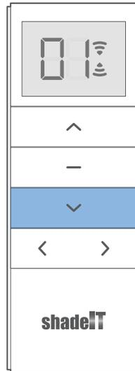
To set the lower limit, hold the down button and let the blind lower. When it gets close to the bottom, press the stop button. Press the down button repeatedly to jog the blind down until the bottom bar rests on the ground. Press and hold the down and stop buttons together until the blind jogs again to acknowledge the lower limit point.
