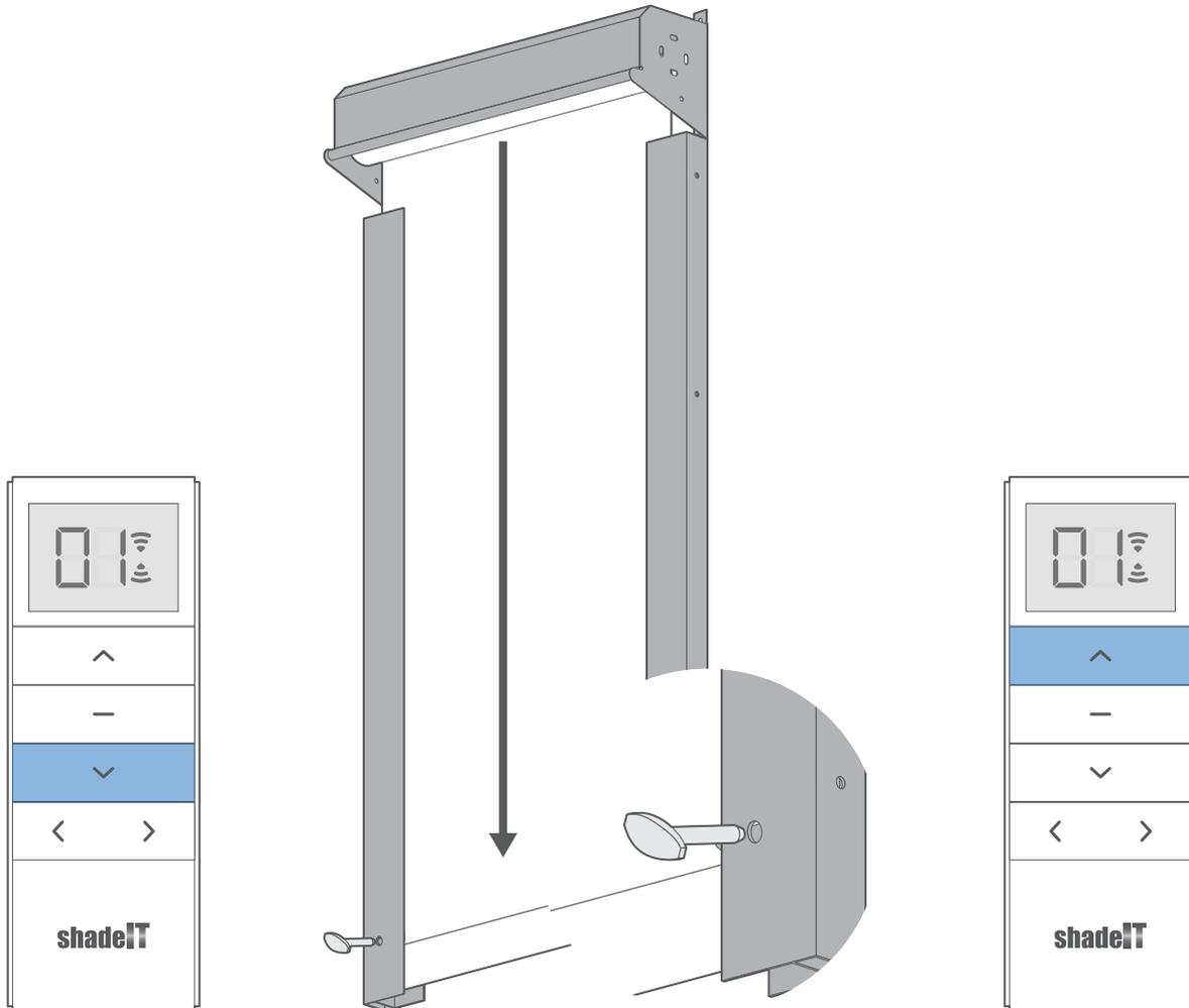
Use the remote to lower the blind. Allow it to lower until it reaches the lower limit point you set before.
