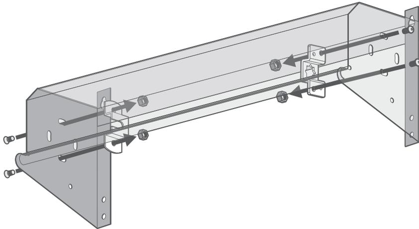
Mount the roller plates to the inside of the cassette, as shown. Use 2 nuts and bolts per plate.
