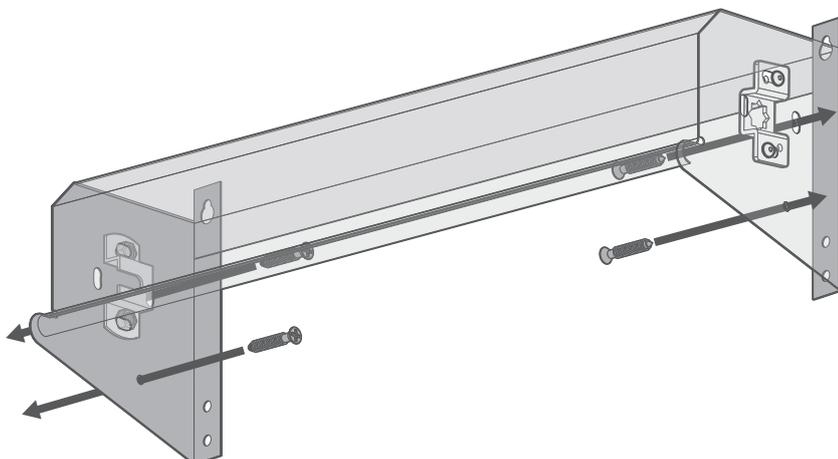
Use 4 screws to mount the cassette to the inside walls of the recess. The cassette will be the 'cover' for the blind.
