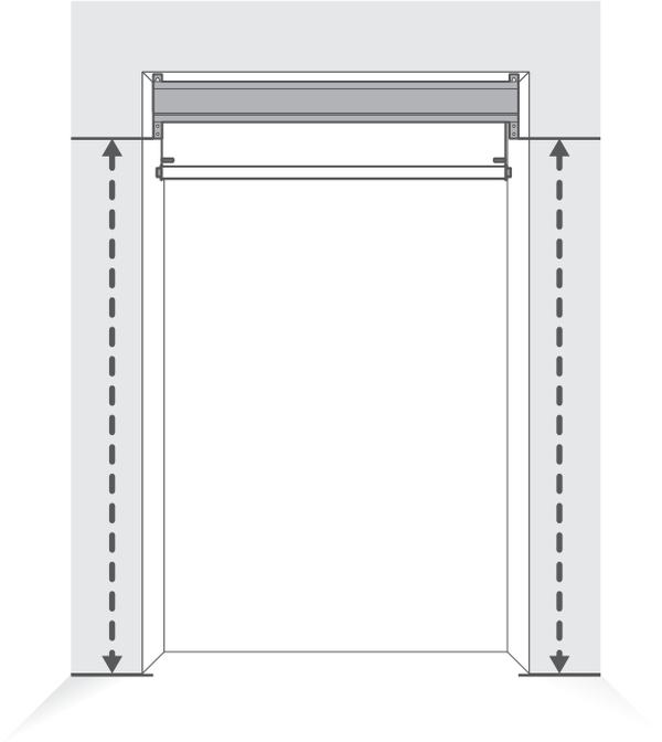
The side channels are provided to you longer than the drop you ordered, so that they can be trimmed to the perfect length. Measure for this by measuring up from the ground to the lowest edge of the cassette.
