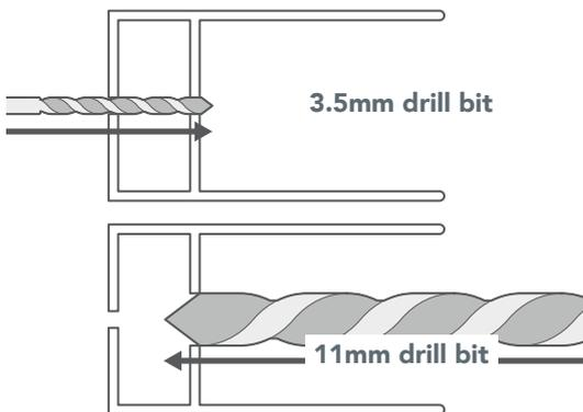
Now, drill a hole through the side channels at each mark.
