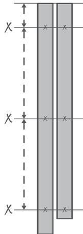
Take these measurements and make matching marks on the insides of your side channels, being as accurate as possible with your measurements.
