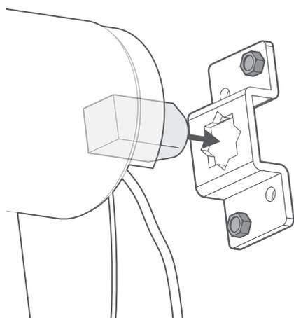
Now raise the blind up into the cassette and slot the square 'peg' on the motor side into the star-shaped slot in the roller plate.
