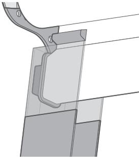
Take the side channels and feed the caps on the blind's bottom bar into the tops of the channels. Hold the channels in position and check them with a spirit level to make sure everything's straight.
