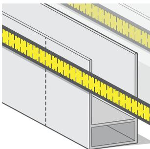
Mark the measurements out on the side channels, being sure to mark the correct channel with each.
