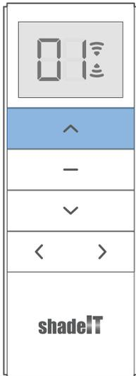
Use the up button to raise the blind until it's close to where you want your upper limit to be, then hit the stop button. Press the up button repeatedly until the blind is exactly where you'd like. To set the upper limit, press and hold both the up and stop buttons together. The blind will 'jog' a couple of times to acknowledge that the stop point is set.
