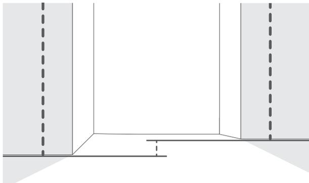
Make sure you measure each side separately, as the ground may be uneven, making one side higher than the other. Make a note of each length measurement.
