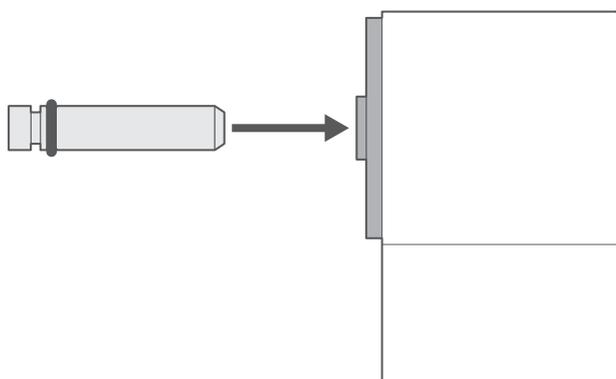
Start by inserting the roller 'pin' in the end of the blind opposite to the motor side. Note that the rubber 'O' ring on the pin should be resting inside the innermost of the two cutout sections.
