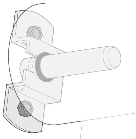
Raise the other end of the blind and slot the roller pin forward into the slot on the other roller plate. Insert the R clip by pushing it up into the holes on the side of the roller plate.
